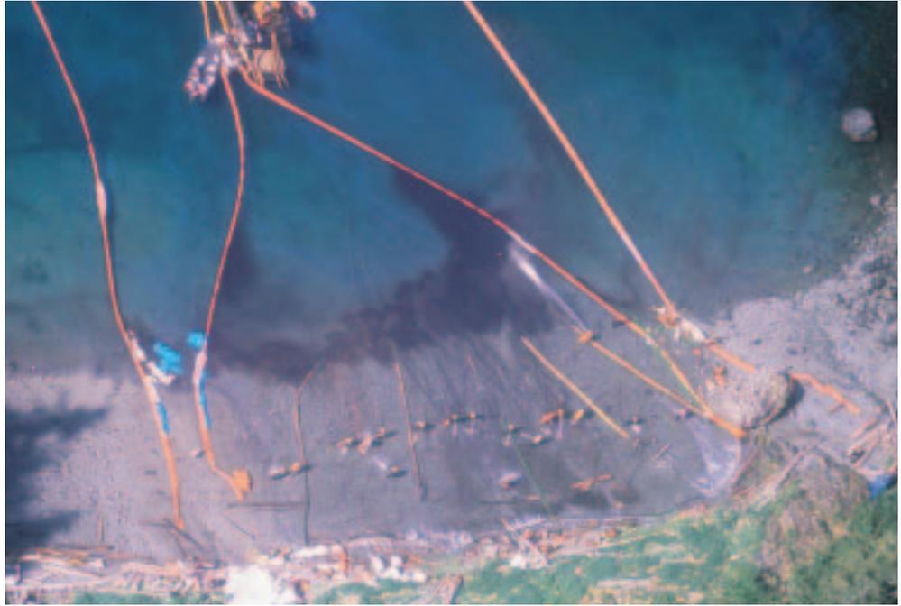
**Figure 3.13** An oil spill can cause short-term changes in populations of aquatic organisms. Toxic chemicals can kill fish and other organisms. In this aerial photo, you can see large, floating barriers called *booms*. They are used to keep the oil from spreading.
