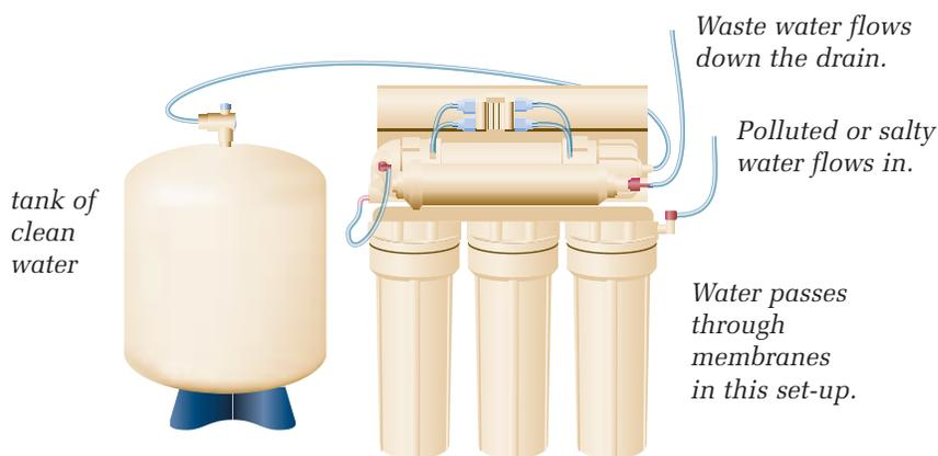
**Figure 1.10** This reverse osmosis set-up can also create pure water from salty or polluted water.
