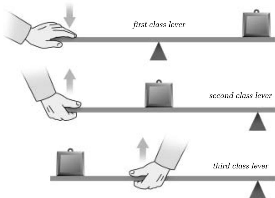
**Figure 1.6** Different ways of using a lever
