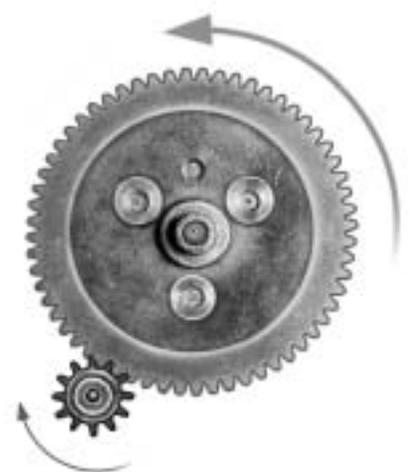
**Figure 1.29** Reducing gears decrease turning speed in a device.
