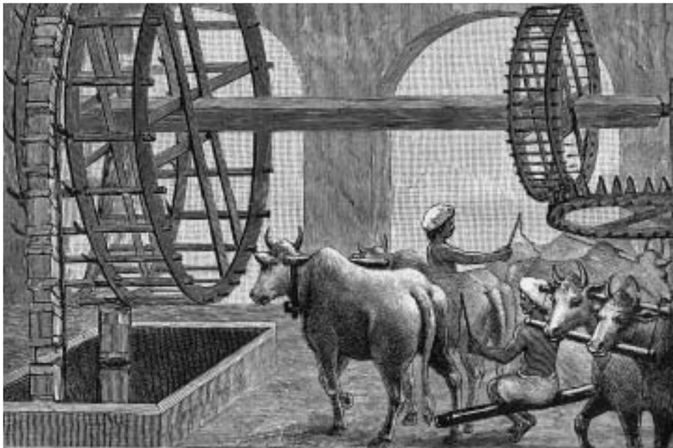
**Figure 1.2** A sakia can be used to haul water out of a well for storage in large tanks or for irrigation.
