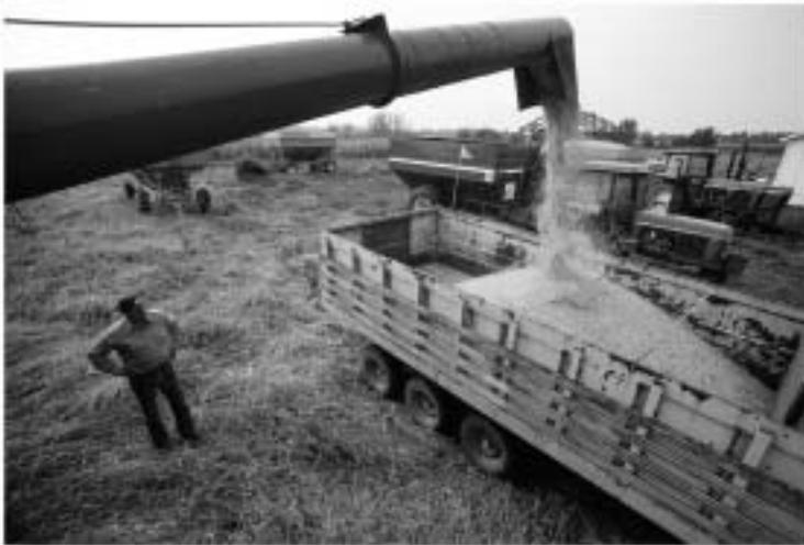
**Figure 1.4** The spiral motion of the slowly turning screw moves the grain into the truck.
