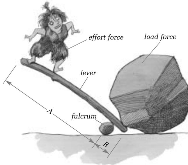
Levers can be labelled in three different ways, according to the location of the fulcrum and the load being moved. Figure 1.6 shows the three kinds or classes of levers. A *first class lever* has the fulcrum between the load and the point where the effort is exerted to move the load. A *second class lever* has the load between the effort and the fulcrum. A *third class lever* has the effort between the load and the fulcrum.
