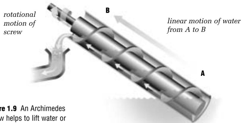
**Figure 1.9** An Archimedes screw helps to lift water or other materials.
