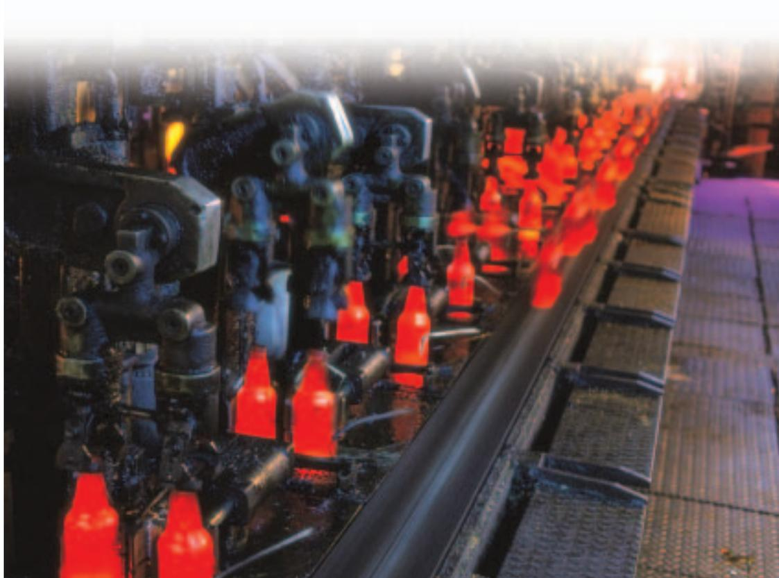
**Figure 1.7** Glass bottles being formed
