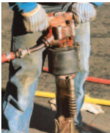
**Figure 1.11** This jackhammer is pneumatic. Systems that use compressed air are called **pneumatic systems**. **Hydraulic systems** use liquids to lift or move things. You will learn more about pneumatic and hydraulic systems when you learn about the compression of fluids in sections 3.0 and 4.0.
