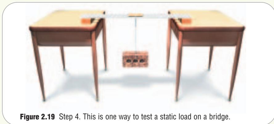
**Figure 2.19** Step 4. This is one way to test a static load on a bridge.
